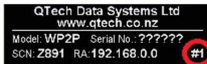
There are ten individual frequency bands referred to as *Channel Numbers* allowing up to ten WP2P systems to be used in the same area. The Channel Number is identified by the “#” on the packaging label; this example is “Channel #1”.
