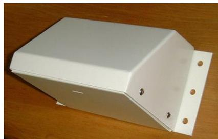
Figure 1: WDL in rugged enclosure (antenna version not shown)
