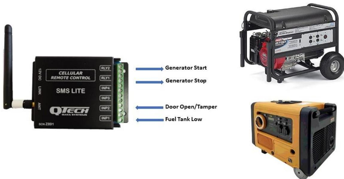
There are many different types of generators available, but you need to ensure that yours is fitted with a suitable electrical interface for remote starting.
