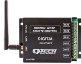
Earlier revision WP2P modules, with white printing, can be used in the same MPC system as Revision E WP2P module but a firmware upgrade is required. This upgrade can only be performed at QTech. Please contact us for further details.
