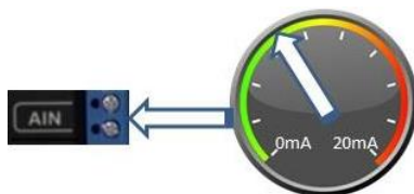
WP2P Module 1 Analogue 0-20mA signal input
