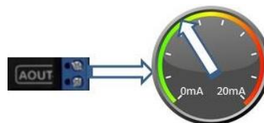
WP2P Module 2 Analogue 0-20mA signal output
