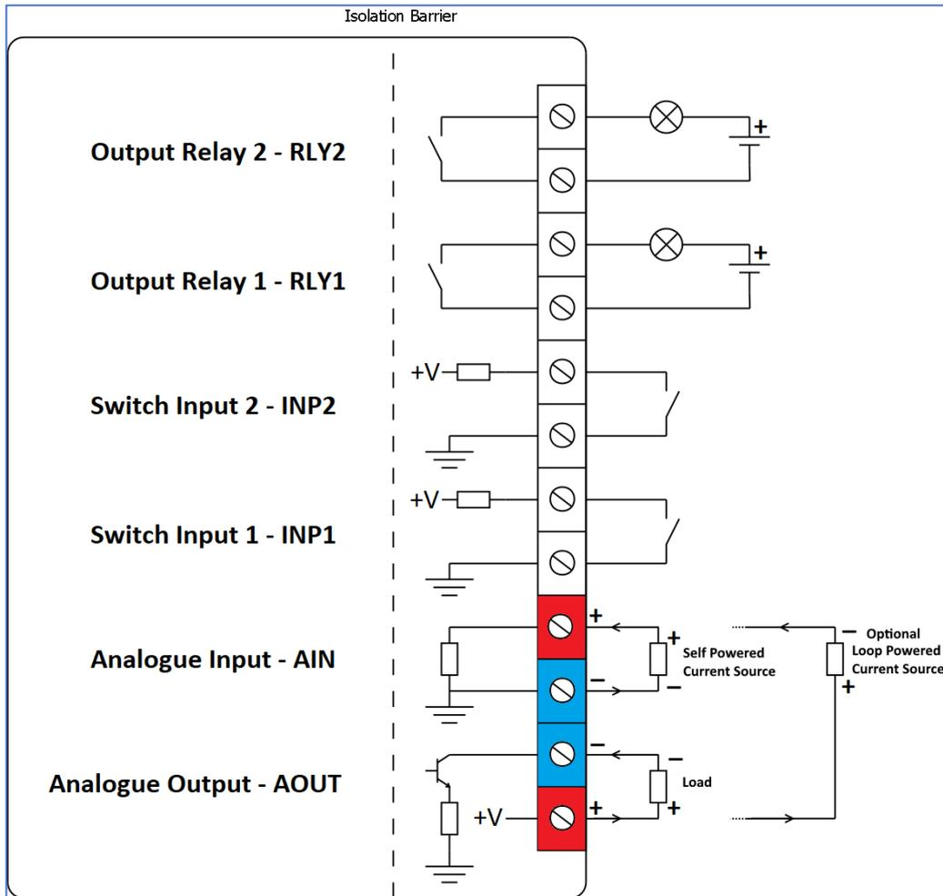
Figure 3. Input Output Wiring Diagram
