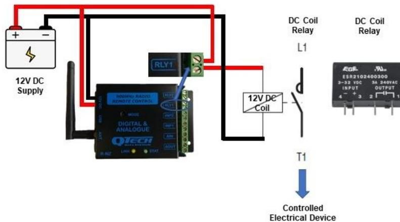
Figure 2. Interface Relay – Typical Wiring Diagram
