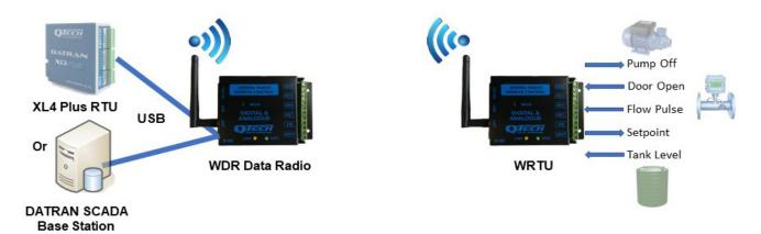
WRTU modules are available with digital I/O (WRTU-D) or digital plus analogue I/O (WRTU-DA), allowing you to transmit 4-20mA sensor readings as well as remotely control electrical devices. For example, a WRTU-DA can provide water level information and turn pumps on and off from the DATRAN VI SCADA user interfaces.
